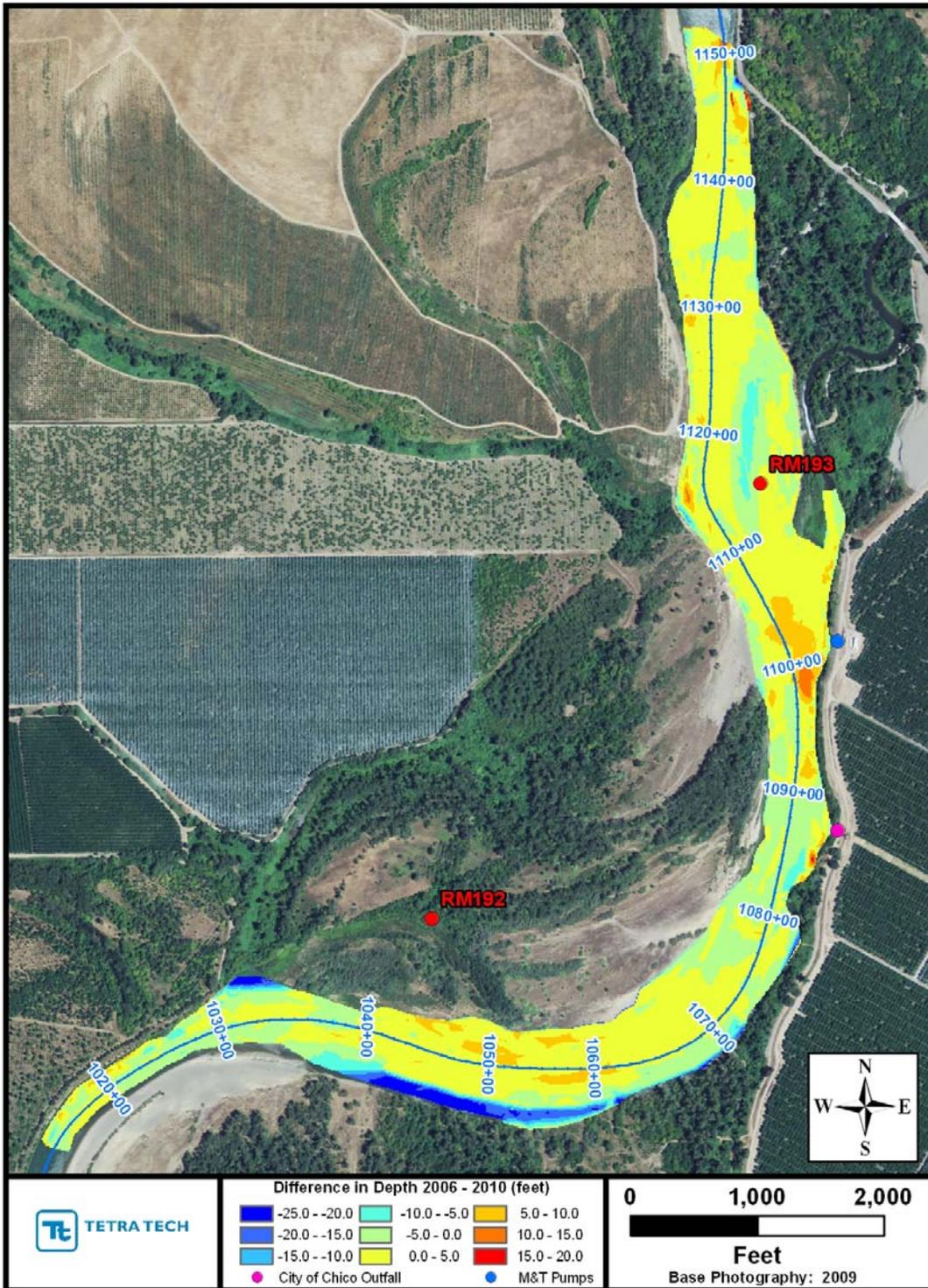
Figure 3. Isopach map of differences in channel topography between 2005/2006 and 2010 surveys.
