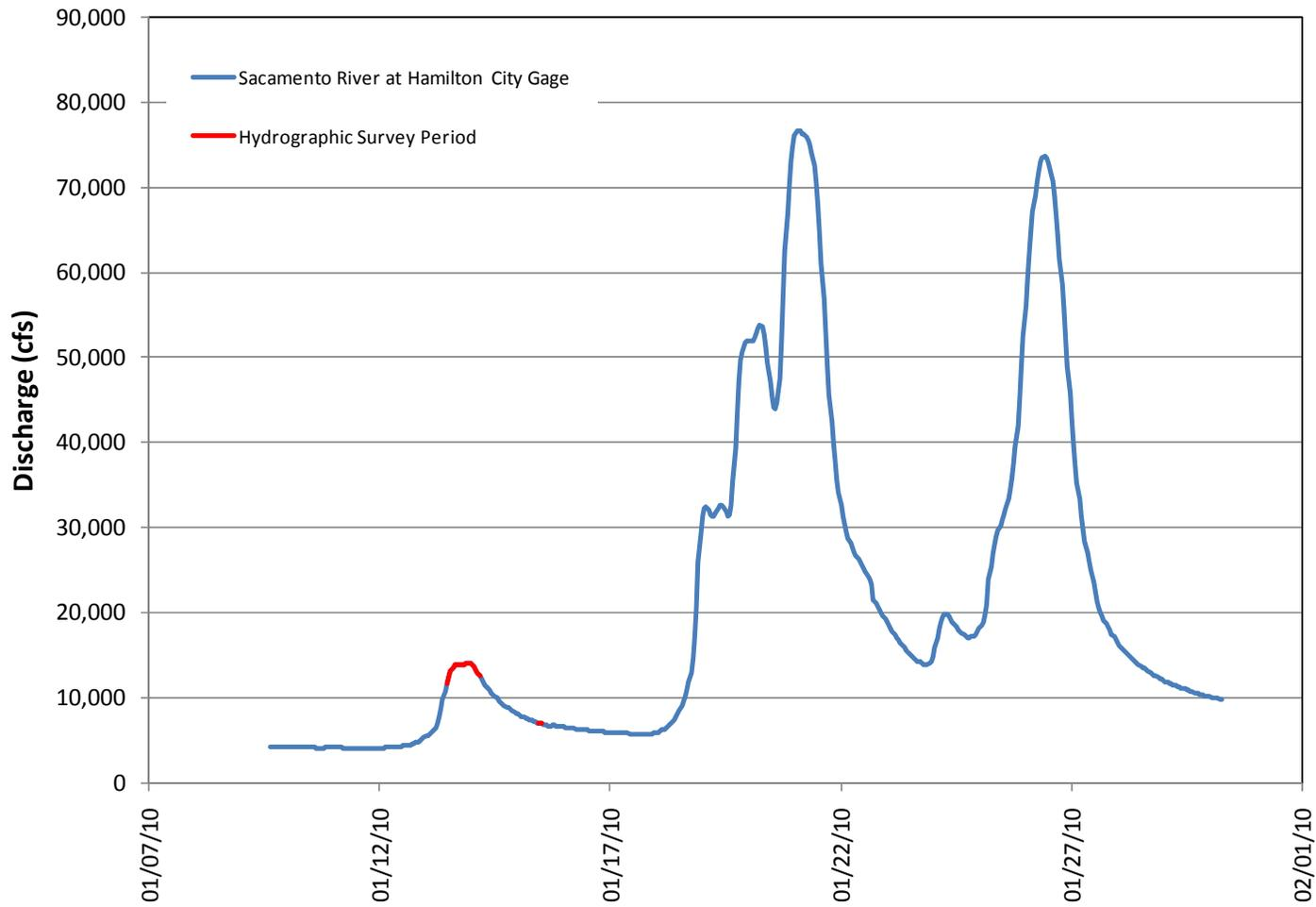
Figure 1. Hamilton City gage flows during and after the January 2010 bathymetric survey.
