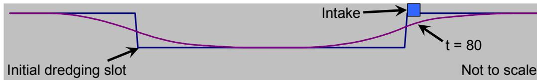
**Figure 2. Simulated results, showing changes in bed elevation, as a demonstration of the functionality of dredging gravel bar upstream of the intake.**
