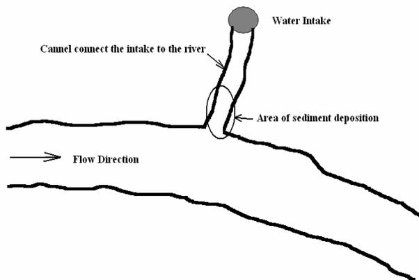
**Figure 1.** A schematic diagram of a water intake connected to the main water body with a cannel. The oval indicates the primary area of sediment deposition that may need to be frequently dredged.
