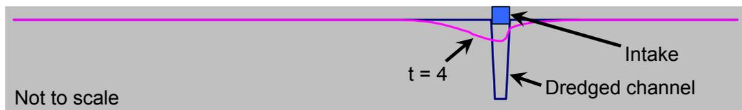
**Figure 3. Simulated results, showing changes in bed elevation, as a demonstration of the fluvial process following the dredging of a channel toward the intake.**
